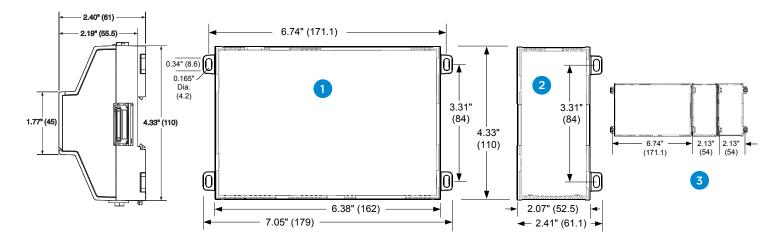
Compatible with (DIN43880) enclosures Suitable for mounting to a panel or to an EN50022 standard 35mm rail
